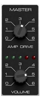
**Amp Drive**- Because a big part of overall Polivoks character comes from its voltage-controlled amplifier (VCA) section, we've modeled and included it in the Master section. The VCA is essentially "open" all the time, but the Amp Drive knob sets its level of distortion drive.
