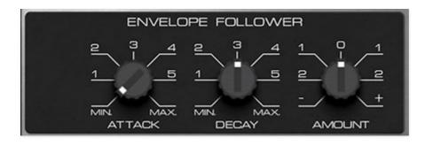
**Attack**- Defines the length of time for cutoff to rise from minimum to maximum when an input signal is detected.
