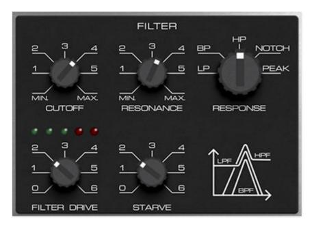
**Cutoff**- Sets the frequency where frequency attenuation begins. Its effect is dependent upon the currently selected filter *Response* setting.
