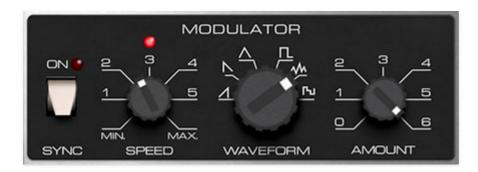
**Sync**- When the *Sync* switch is enabled, Modulator speed will lock to host tempo when using Atomika within DAW software, or to the current tempo in the top menu bar when using the standalone version.
